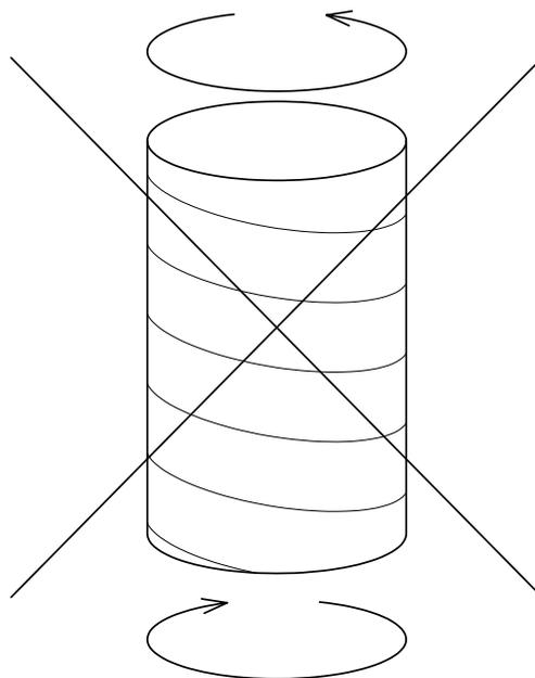
Axial torsion, bending loads and deviation from the axis must be avoided.
