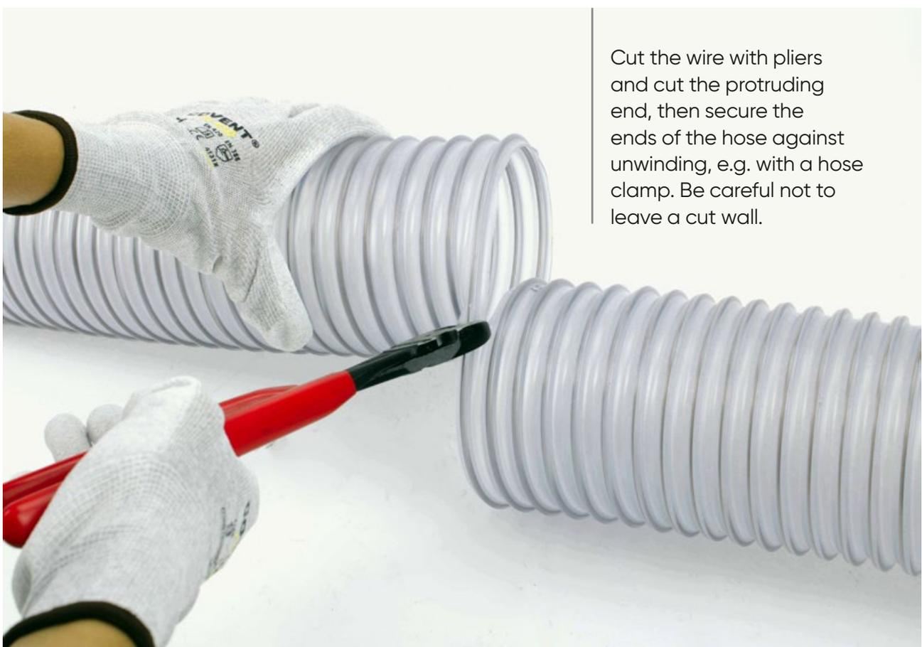
Cut the wire with pliers and cut the protruding end, then secure the ends of the hose against unwinding, e.g. with a hose clamp. Be careful not to leave a cut wall.
