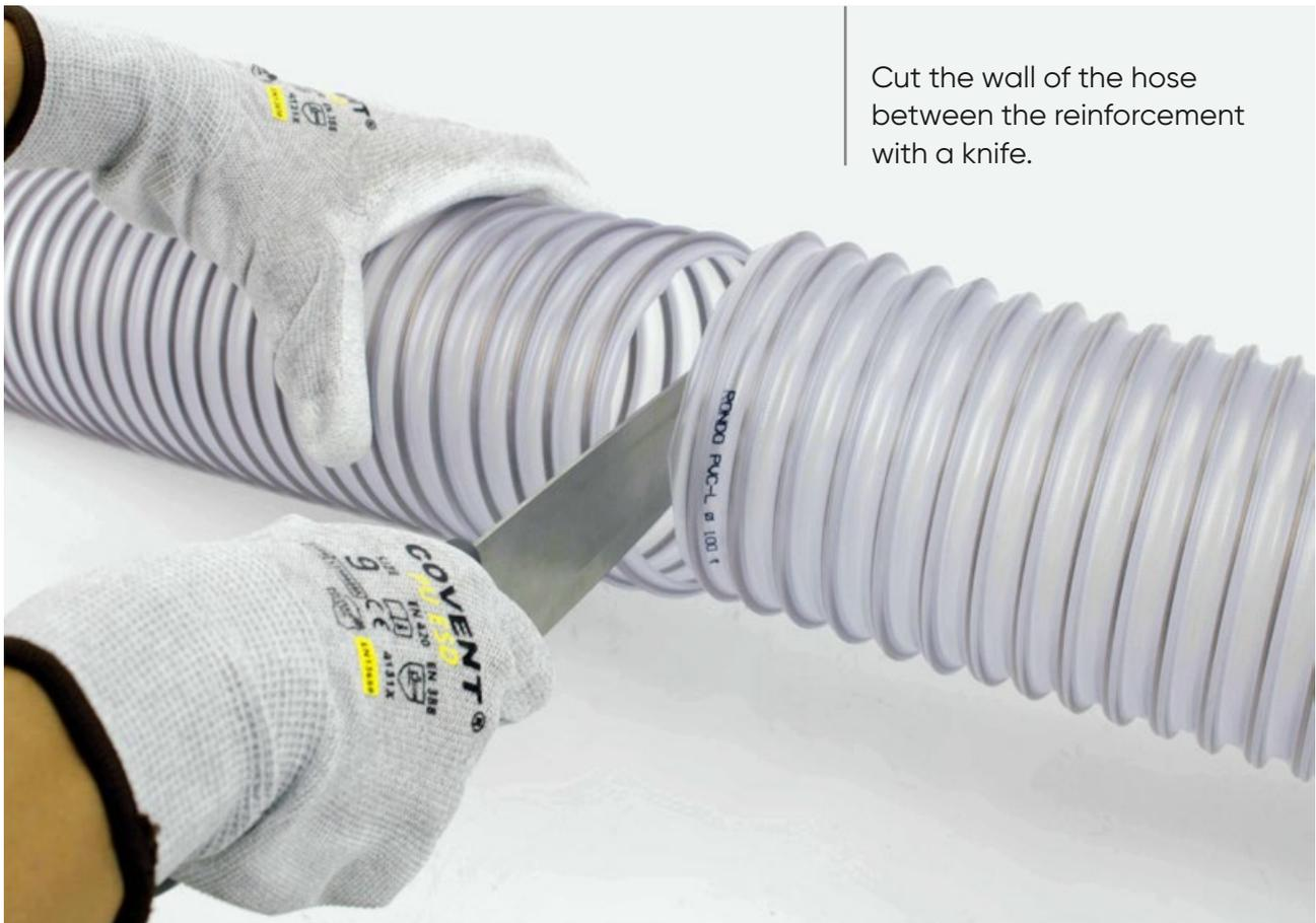
Cut the wall of the hose between the reinforcement with a knife.
