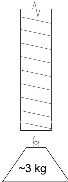
When hanging the hose vertically, the distances between the fixing points should be arranged so that the load does not exceed 3 kg per fixing point (applies to KLIN hoses).
