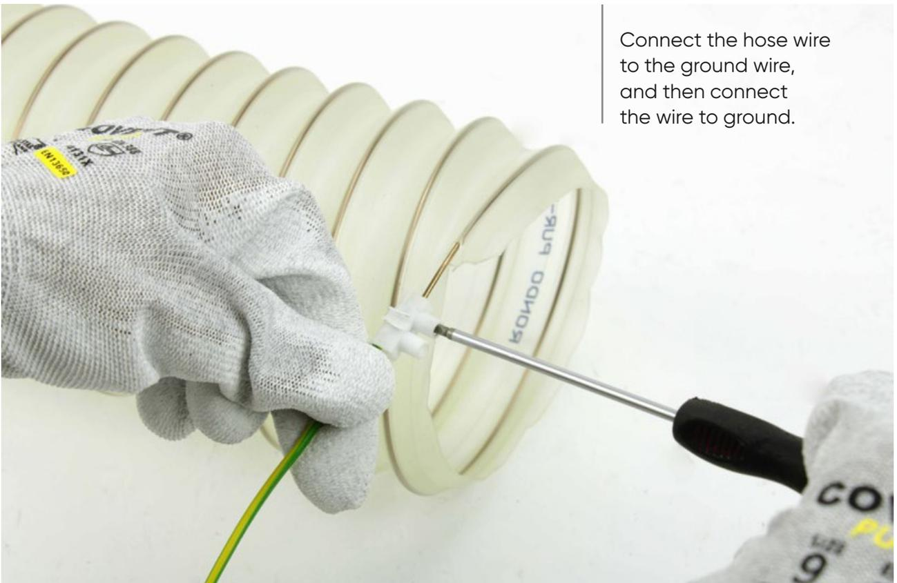
Connect the hose wire to the ground wire, and then connect the wire to ground.
