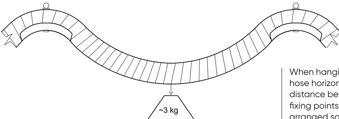
When hanging the hose horizontally, the distance between the fixing points should be arranged so that the load does not exceed 3 kg per attachment point (applies to KLIN hoses).
